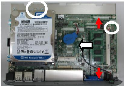
3. Unfasten the HDD screw (x1) and remove the
