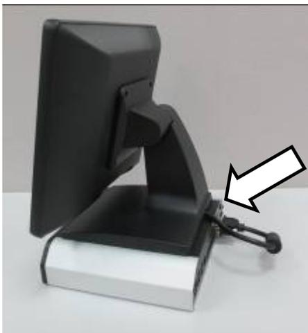
5. Connect the VGA cable to the system.
