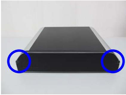
2. Unfasten the screws (x2) to separate the front plate.
