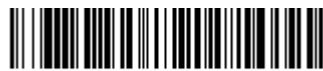
POSTAL25. Planet Code, Postal-4i, and Postnet with B and B' Fields On
